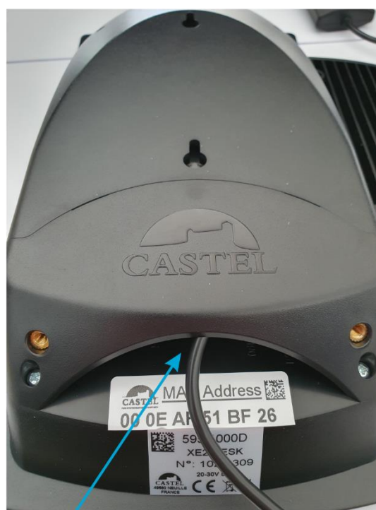
Cord entry into the station
